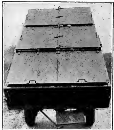
A STANDARD GARBAGE BODY FITTED WITH COVERS
